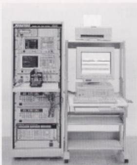
<R2122C/S Power Amp. Test System>
